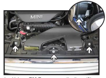
Using a T30 Torx, remove the three (3) screws from the top edge of the fascia. Then remove the two (2) screws next to the headlights, there is one (1) on each side (inset).
