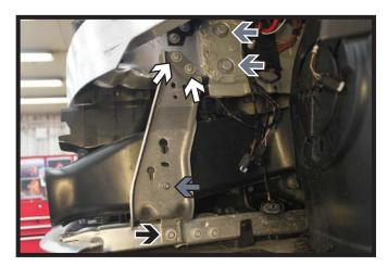
7. Using a T30 Torx, remove the two (2) screws from the top of the support bracket (white). Using a T25 Torx, remove the screw from the duct (gray). Using a 8MM socket, remove the bolt from the bottom of the support bracket (black).
