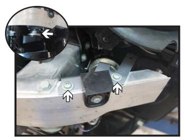
Leaving the lower horn loose, reinstall the bracket to the vehicle. After the bracket is reinstalled reattach the lower horn to the bracket.
